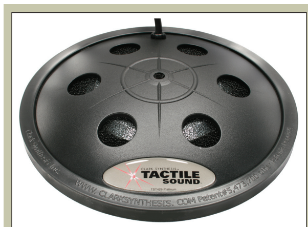
Figure 3. Shakers are very low frequency subwoofers that transduce sound energy in the 50 Hz to 150 Hz range. They are typically bolted to the seat of the drummer or placed on the floor near the bass player. Photograph courtesy of Sensaphonics, Inc.
